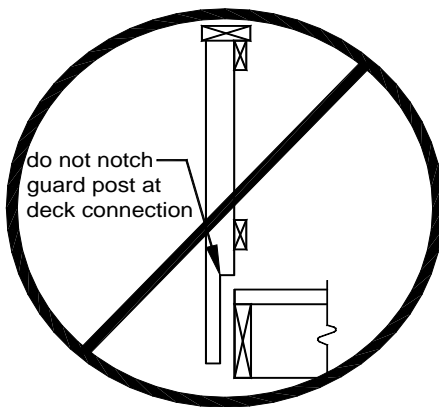
FIGURE 28: NOTCHING AT GUARD POSTS
